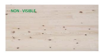
"TROHIS" CLT panels in non-visible quality are perfect for use as load-bearing components which are generally panelled following assembly. Thus, no special requirements on the surface appearance for this quality. Wood grading is always carried out on the basis of strength class C 24. The surface appearance corresponds to appear-ance class C, in accordance with EN 13017-1.
