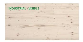
"TROHIS" CLT panels in industrial quality are usually used for industrial buildings with low require- ments on surface quality. Industrial quality is not used for visible surfaces in residential buildings. The lamellae are sometimes finger-jointed, depending on the orientation of the covering layer. The surface is planed and fully smoothed. The surface appearance corresponds to appearance class B, in accordance with EN 13017-1.
