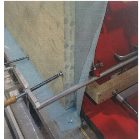
Fig. 1: Test specimen 1, 60mm, 3-ply with airtight sealing and foil for reference measurement
